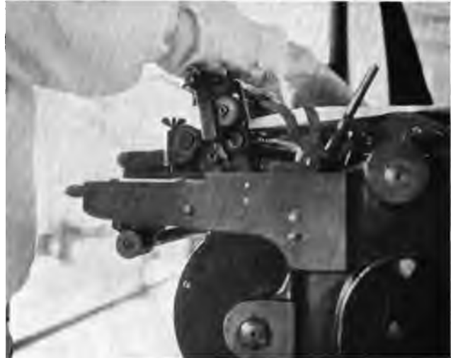
Fig. 2. Gear Accident at Feed Rolls.
